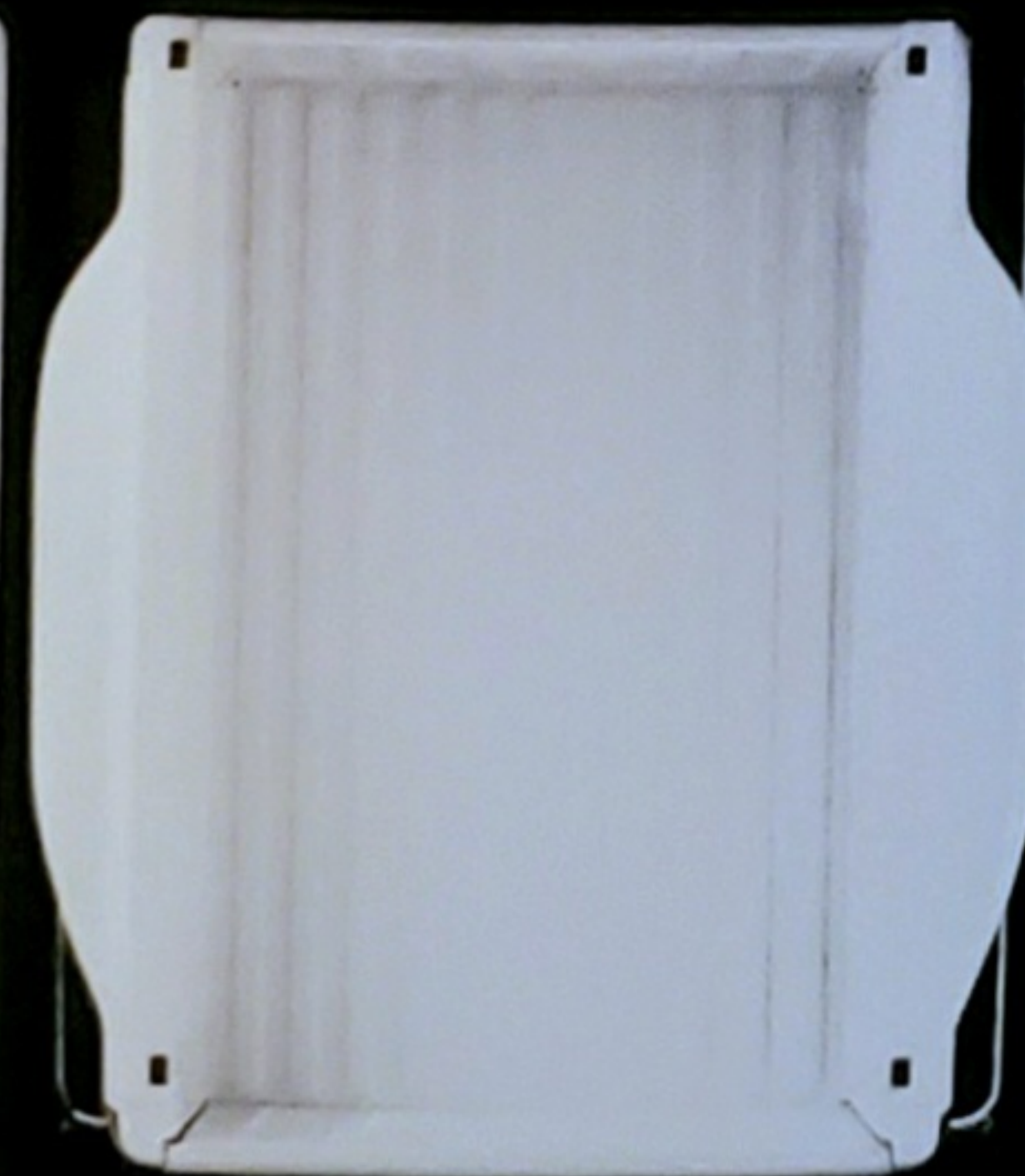
SPORTSIDE BED LENGTH: 78.7" X WIDTH: 49.1" WIDTH BETWEEN WHEEL HOUSINGS: 49.1"
