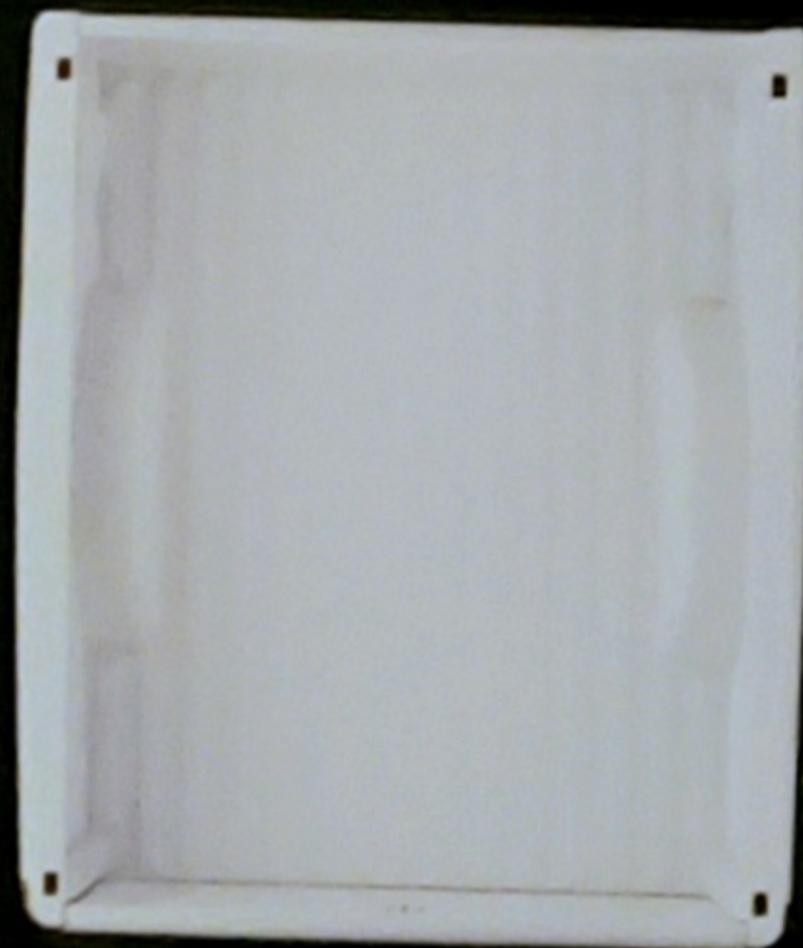
WIDESIDE SHORT BED LENGTH: 78.7" X WIDTH: 64.4" WIDTH BETWEEN WHEEL HOUSINGS: 49.1"
